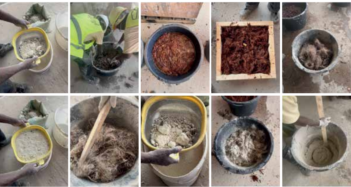
The “coco-crete” ingredients (clockwise): By mixing coral rock - ground into powdered lime stone - with coconut shell fibre (husk) and water, a new building material is formed. Mixing ratio: 1 part lime to 2 ½ parts husk
